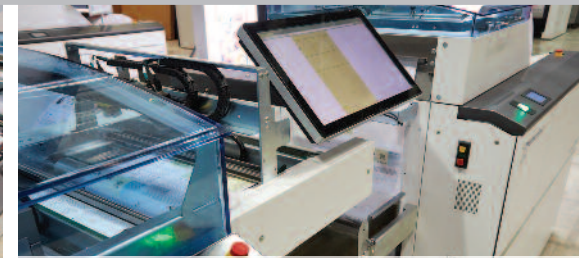
A touchscreen editing tool on the DP8 allows fast and easy set-ups.
